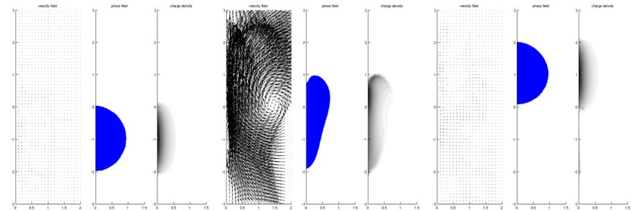
Snapshots of a charged droplet set in motion by switching-off/switching-on of two different electrodes. Depicted are velocity field, phase field and charge density
