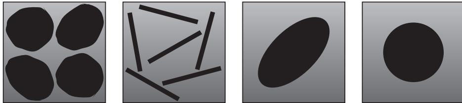
Figure 3.5: Schematic picture of different representative two dimensional unit cells. from left to right: solid phase consisting of several non-connected parts, platy clays (cf. [133]), idealized anisotropic and isotropic material
