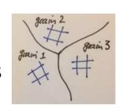
Herring: local balance of surface tensions → angle condition
