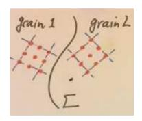
Aging of polycrystals via diffusion-less phase transition reduction of interfacial energy by MCF (Mullins)
